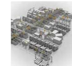
In manufacturing systems, machines and cells are arranged according to the production flow (flow principle), which means they are arranged based on the required operating sequence. The workpiece runs through all processes in synchronized machines. Demand-driven decoupling between individual processes can also be provided (flexible line manufacturing).
